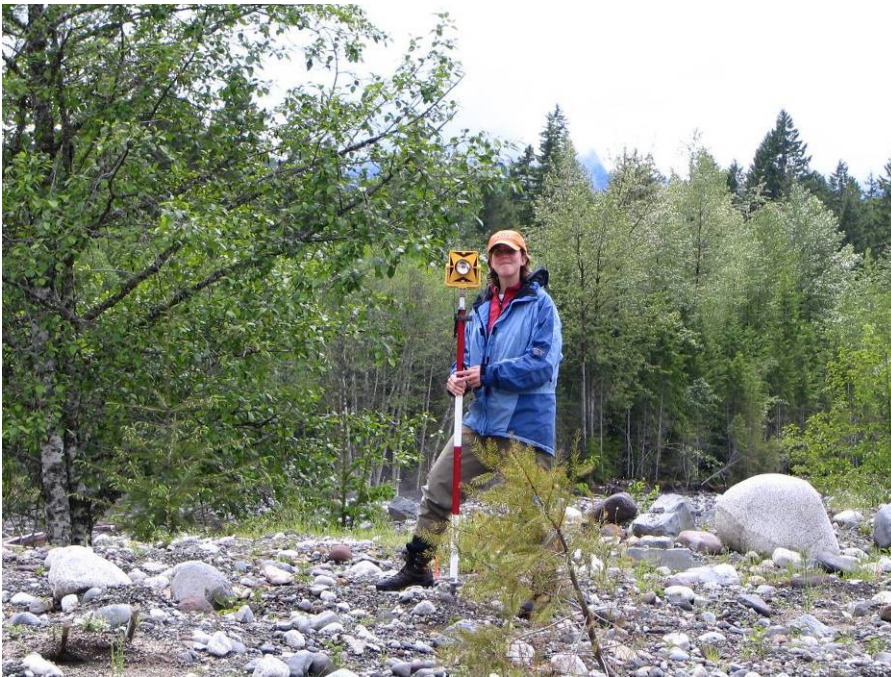
▲ FIGURE 3.2 Prism and adjustable-height rod assembly (Photo: Scott Beason, 6/17/2006).
