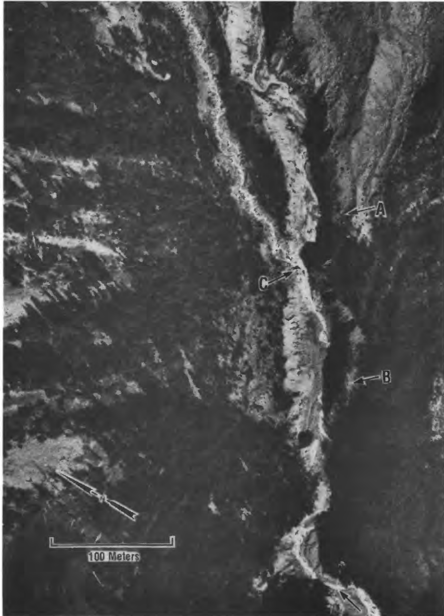
Figure 27.--Vertical aerial photograph taken September 29, 1992 showing regions of bank failure during debris flows of September, 1992 along Tahoma Creek. 'A' and 'B' indicate areas of bank failure, the first such in this reach since 1987. 'C' indicates site of bedrock erosion described in text. Wonderland Trail suspension bridge is at bottom center (arrow). Upstream is towards the top. Scale is approximate. Photograph by Washington State Department of Transportation.
