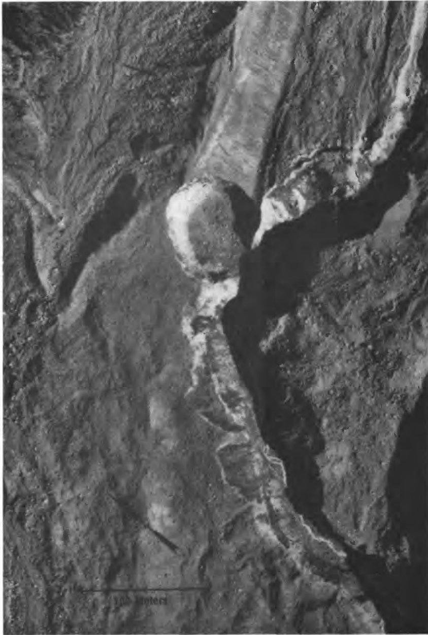
Figure 16.--Vertical aerial photograph taken October 28, 1988 of lower stagnant-ice area along Tahoma Creek, showing scar of slope failure associated with the October 16, 1988 debris flow. Upstream is towards the top. Scale is approximate. Compare to Figure 15. Photograph by Washington State Department of Transportation.
