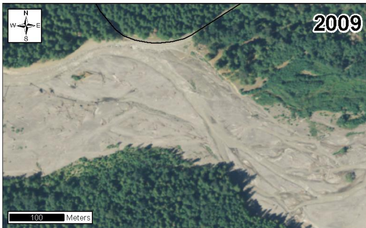
Figure 7: National Agriculture Imagery Program (NAIP) true-color aerial photos from summer 2006 (above) to summer 2009 (below) showing the dramatic change at Sunshine Point Campground due to flood damage on November 6-7, 2006. Approximate bank erosion is 27,540 m 2 (296,500 ft 2 ) (Beason, 2007). Scale: 1:4,109.
