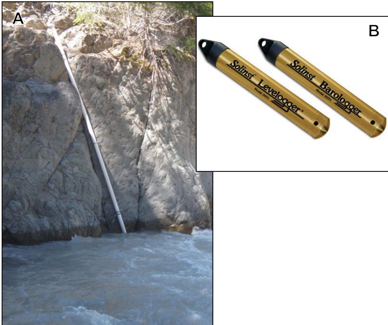
Figure 2: (A) Nisqually River stream gage (stilling well) at Longmire and (B) Solinst® Levelogger® and Barologger® pressure transducers used in this study.
