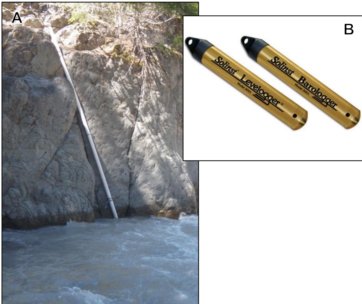
Figure 2: (A) Nisqually River stream gage (stilling well) at Longmire and (B) Solinst® Levelogger® and Barologger® pressure transducers used in this study.
