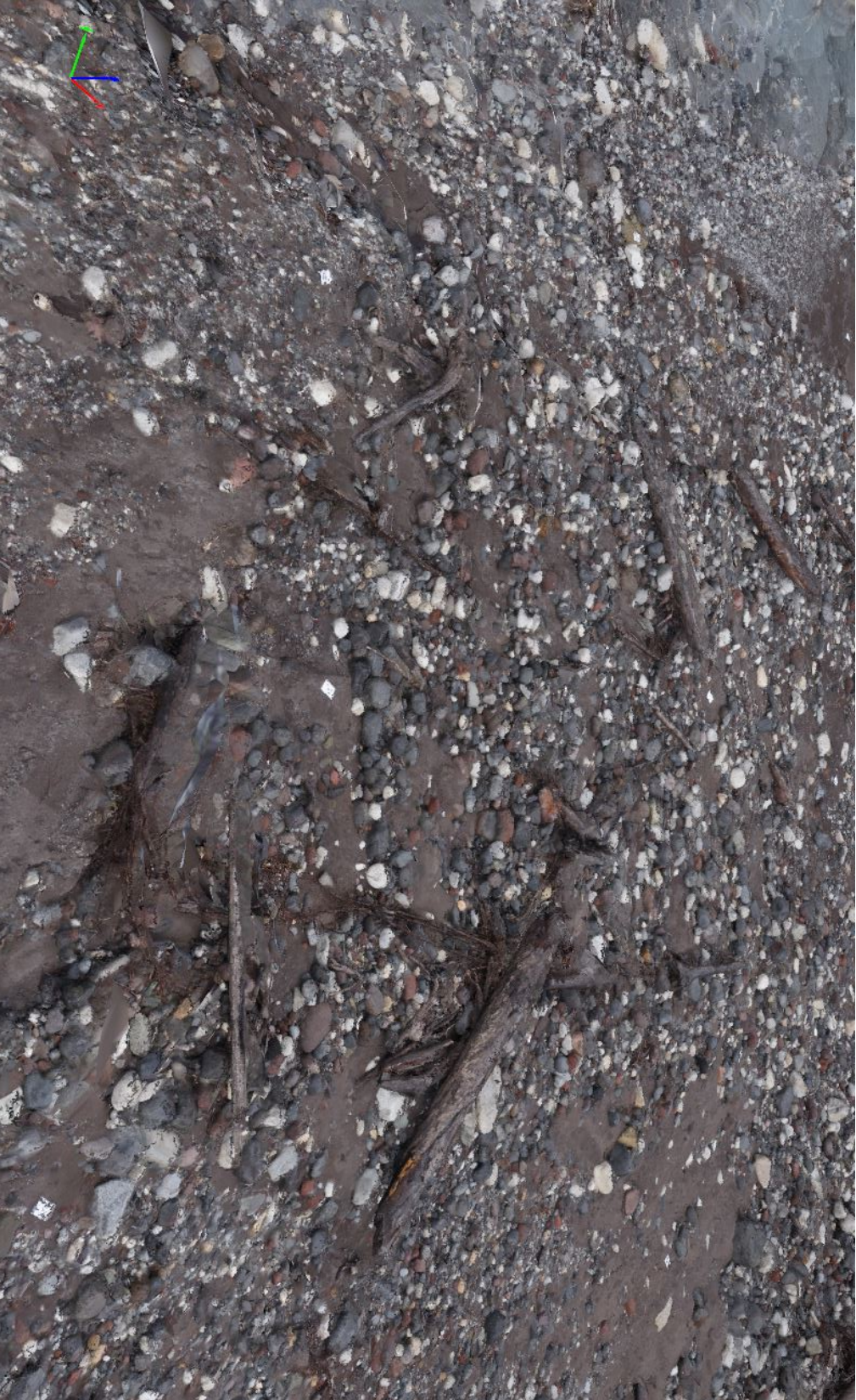
Figure 6: A zoomed shot of the point cloud that was made using Pix4D. Resolution is 10.07 mm/pix. The logs in the photo are approximately 20-25 feet in length.
