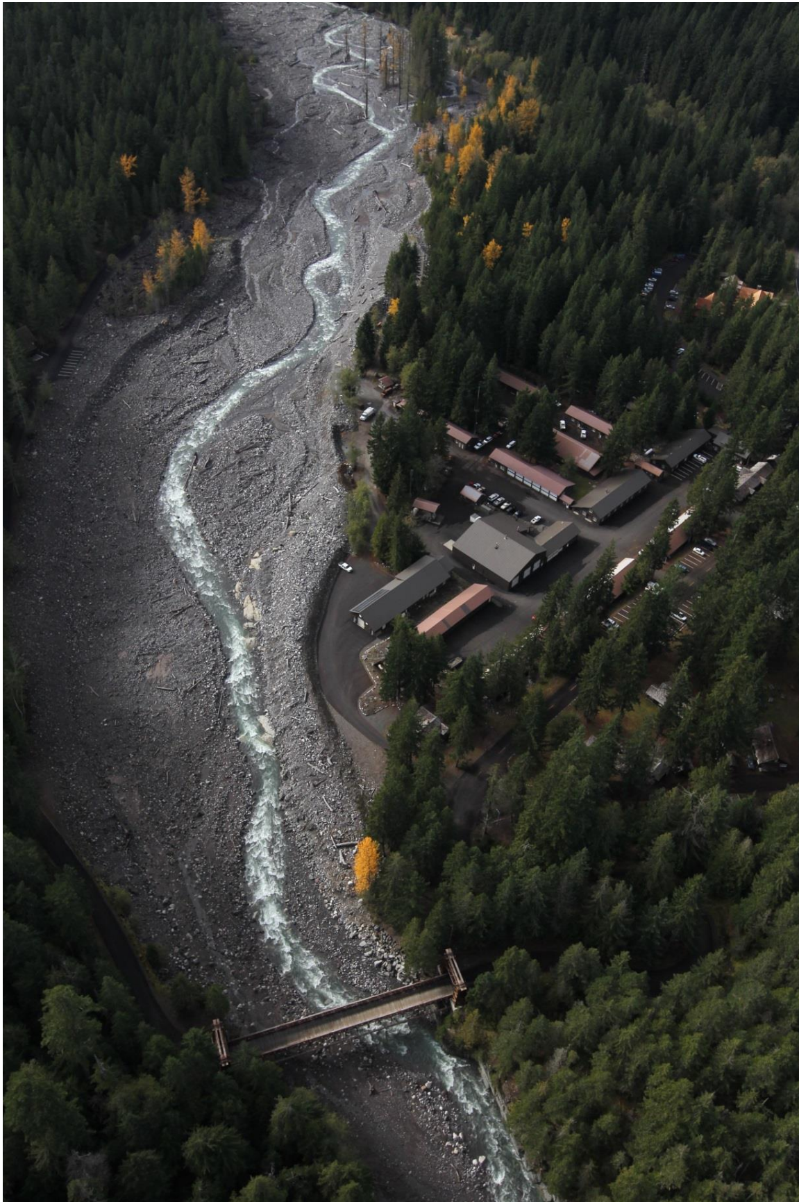
Figure 4: A 2010 aerial photograph of Longmire and the Nisqually River as seen from above. The constructed levee can be seen on the right bank. This photograph shows that the Nisqually is higher in elevation than Longmire itself. (Credit: Dean Koepfler, The News Tribune, Tacoma,
