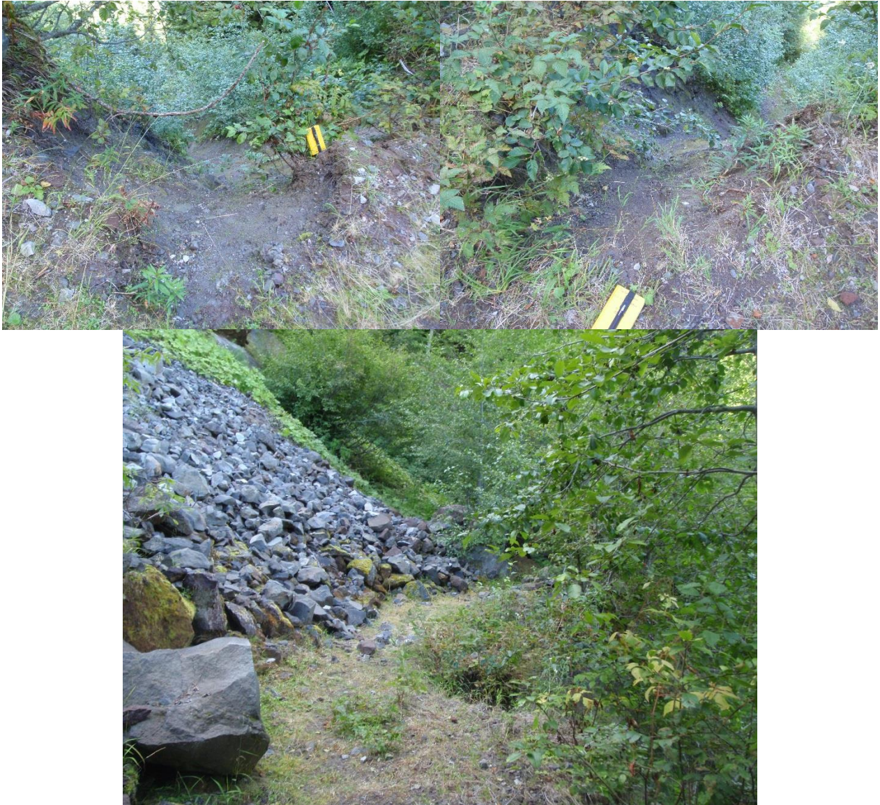
Appendix Figure 5: Point 13 Conditions. Upper left and right photos show the W and E colluvial hollow crowns, respectively. The lower photo is taken from the E edge of the point looking W, and shows the rockfall that contacts the trail.
