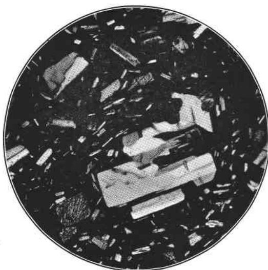
B. Under crossed nicols. (The component parts of the plagioclase phenocryst are, for the most part, arranged in a parallel fashion; however, one side is formed by individual crystals oriented in different directions, indicating a glomeroporphyritic mechanism.)
