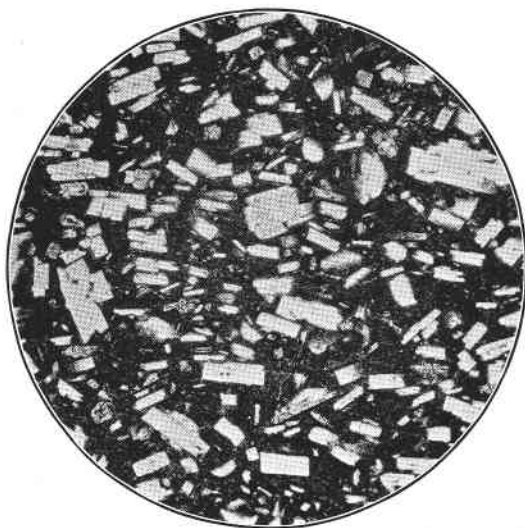
FIG. 20. Andesite from Register Rock at the summit of the mountain. (x25, plane light. It is quite usual for the rocks near the summit to display a well-developed fluxion structure.)
