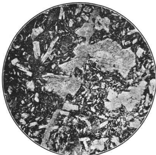
A. Section view. (The larger and more irregular phenocrysts of plagioclase are charged with magnetite dust and flakes of antigorite. A small veinlet of antigorite and titanite may be seen cutting across the rock.)
