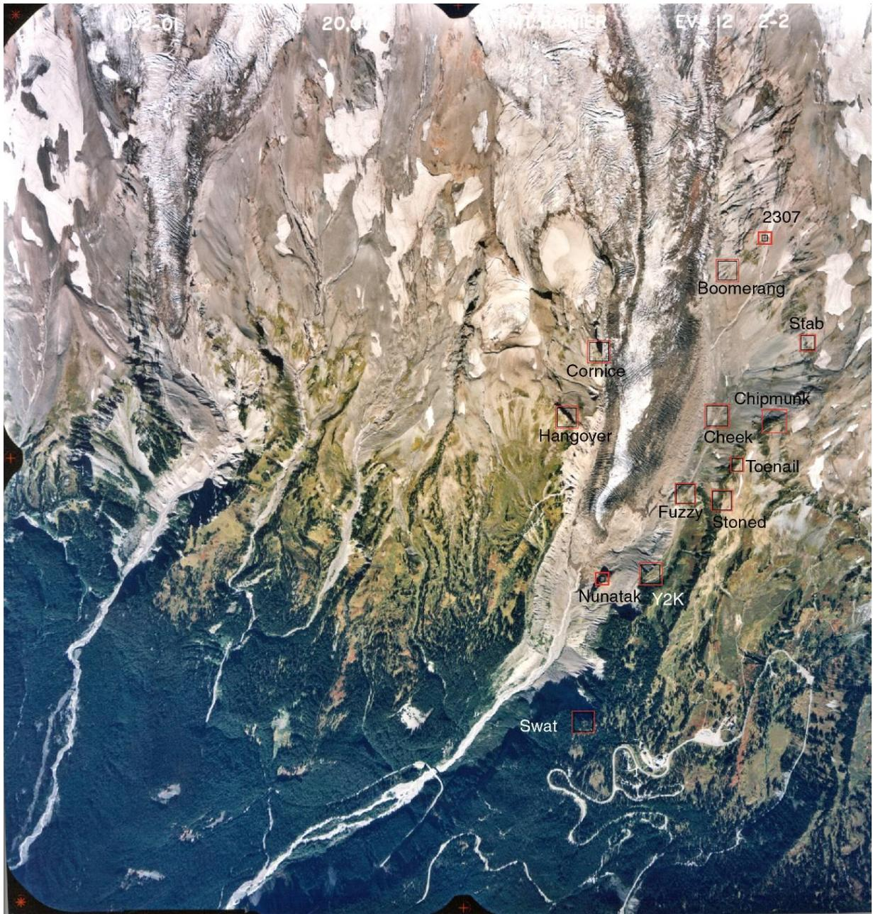
Figure SOP 11.4. Photo identifiable ground control points surrounding Nisqually Glacier.
