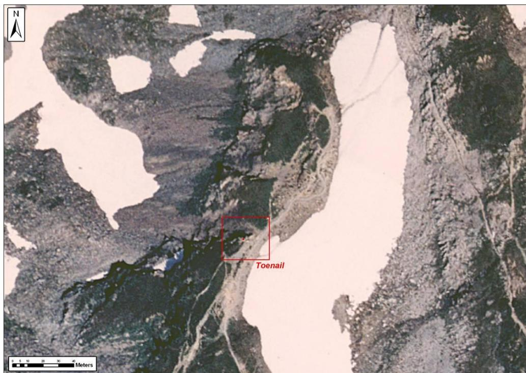
Figure SOP 11.9. Photo identifiable ground control point “Toenail” surrounding Nisqually Glacier.
