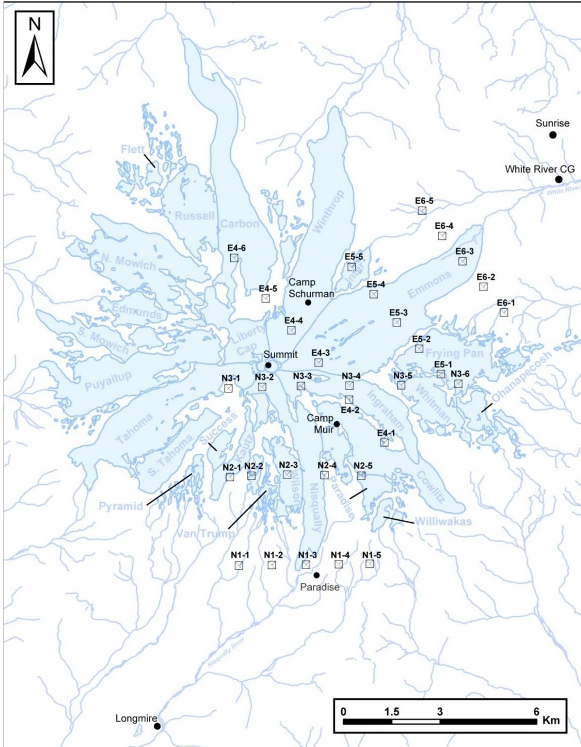
Figure SOP 10.1. Location of air photo centers and flightlines from 2004 flights for Nisqually and Emmons glaciers. Each flightline is at a different elevation to maintain a scale of approximately 1:12,000. The labels in this figure refer to the Photo Labels in Table SOP 10.1 (N is for Nisqually, E is for Emmons).
