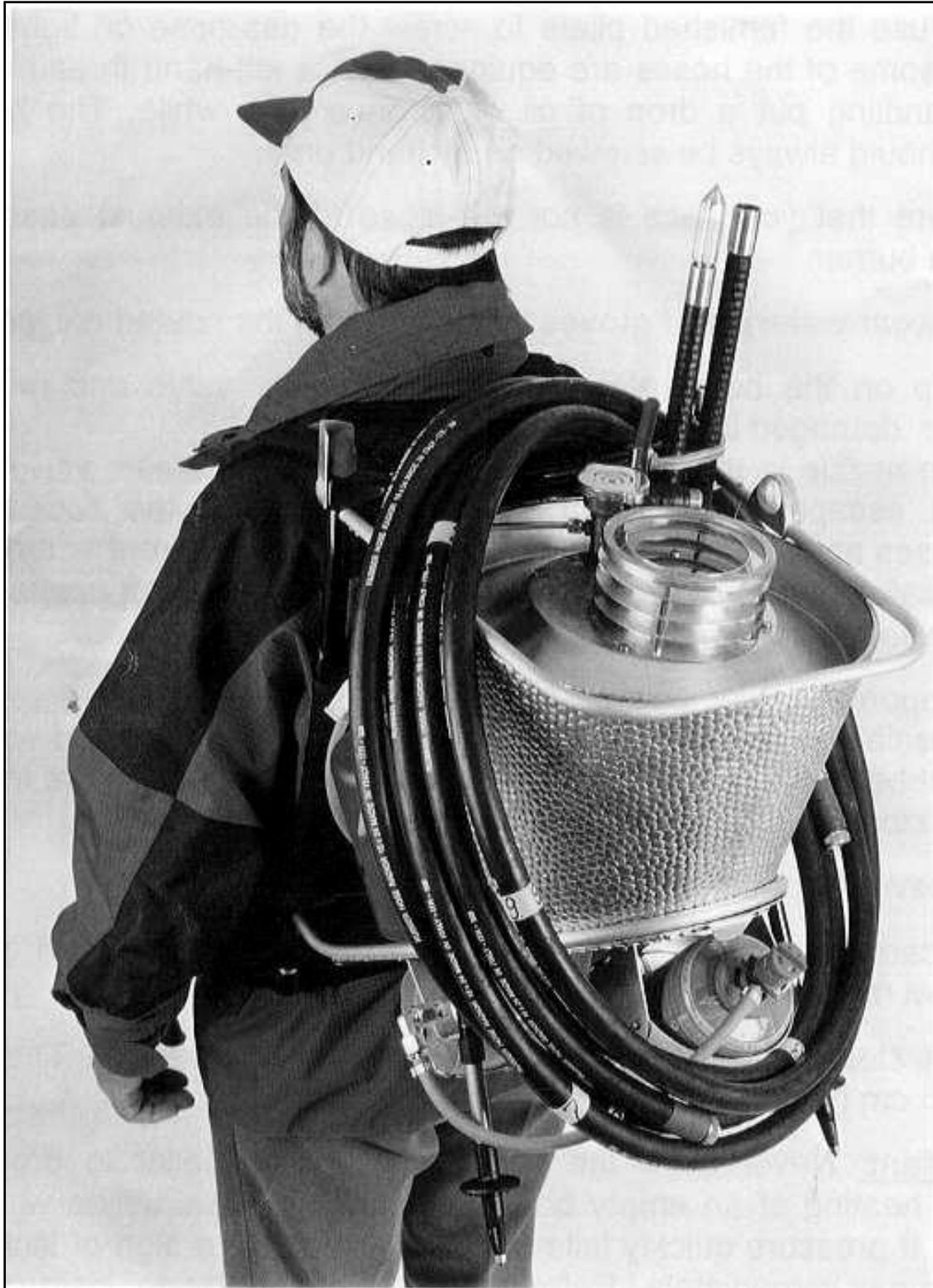
Figure SOP 4.4. Showing the correct way to package the Heucke Ice Drill for field transport.
