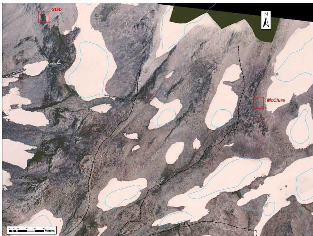
Figure SOP 11.8. Photo identifiable ground control points “Stab” and “McClure” surrounding Nisqually Glacier.
