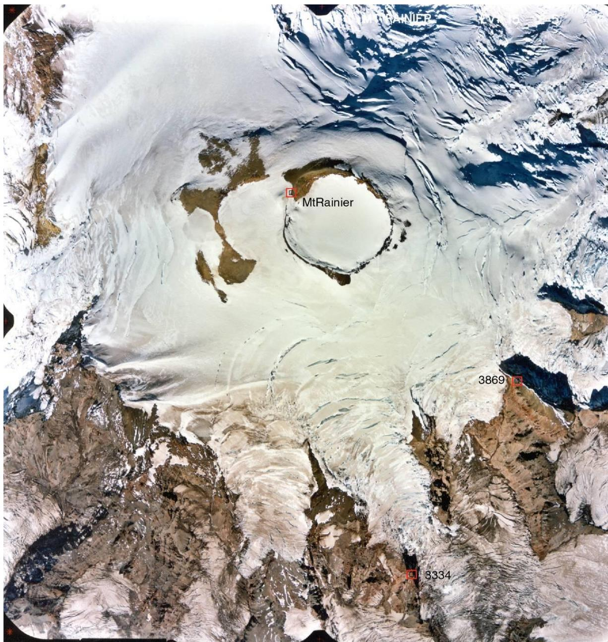
Figure SOP 11.5. Photo identifiable ground control points “Mt Rainier” and “3334” surrounding Nisqually Glacier.
