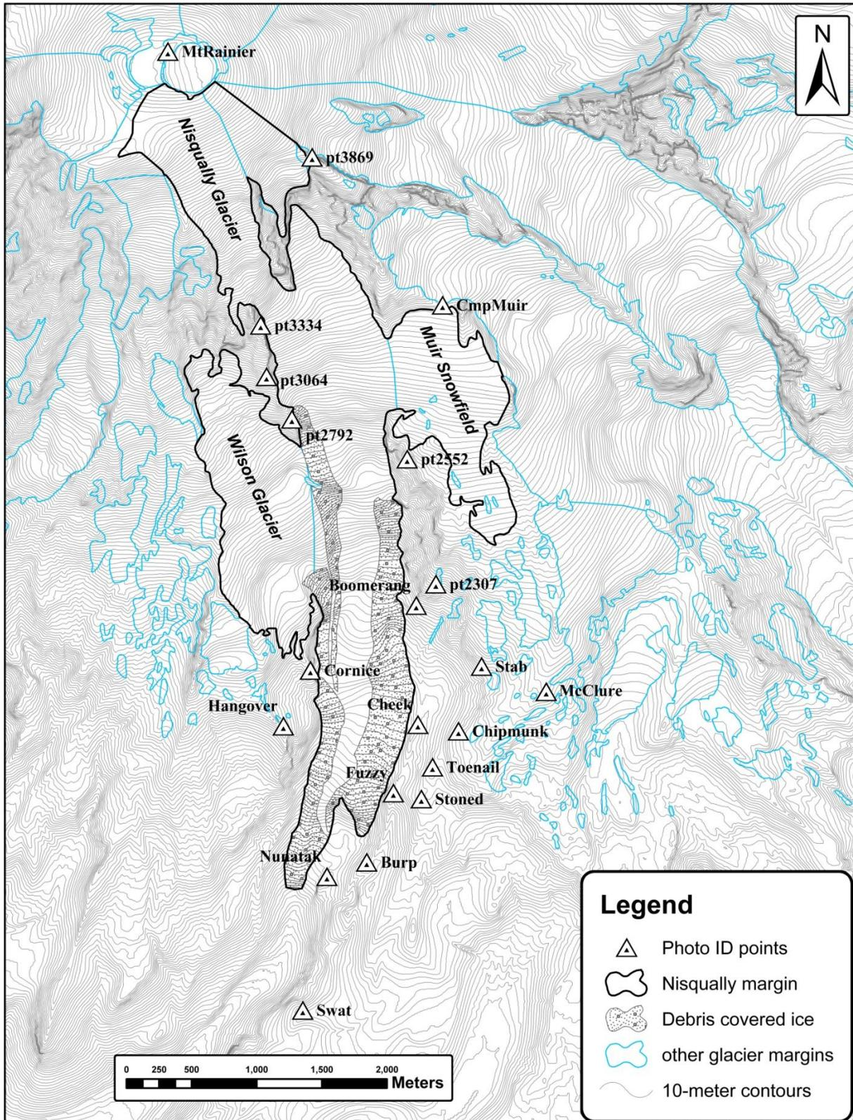
Figure SOP 11.1. Photo identifiable ground control points surrounding Nisqually Glacier.
