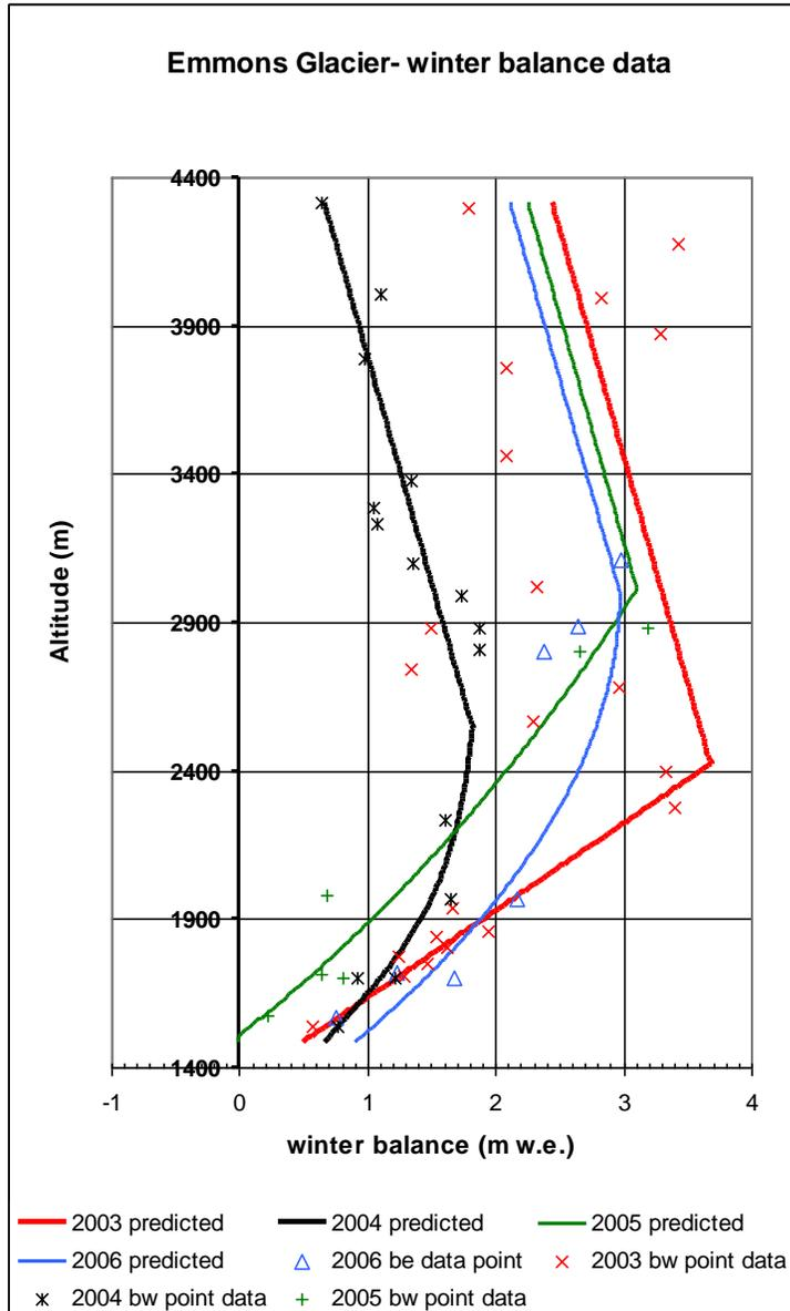
Figure SOP 7.2. Point data and predicted ( $b_w$ ) for all years on record. Note  $b_w$  decreases above a 2,400 and 3,000 m elevation on the glacier.
