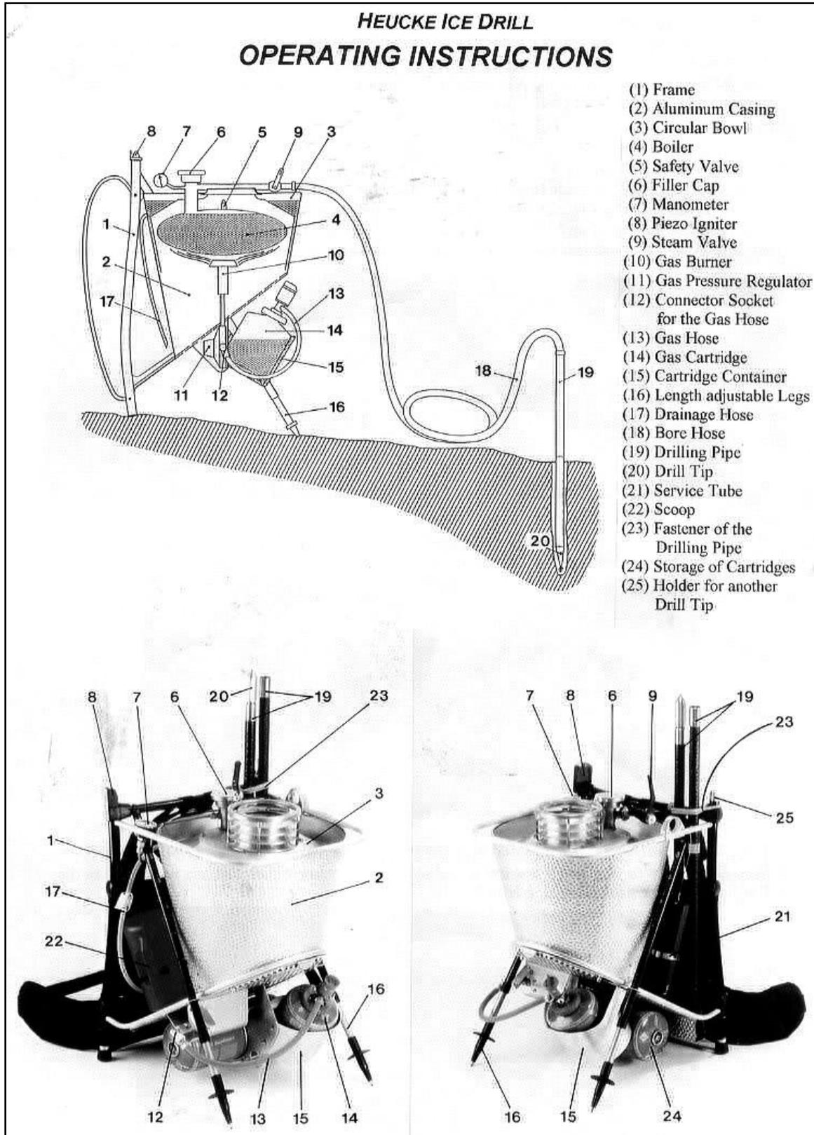
Figure SOP 4.2. Operating instructions for using the Heucke Ice Drill.
