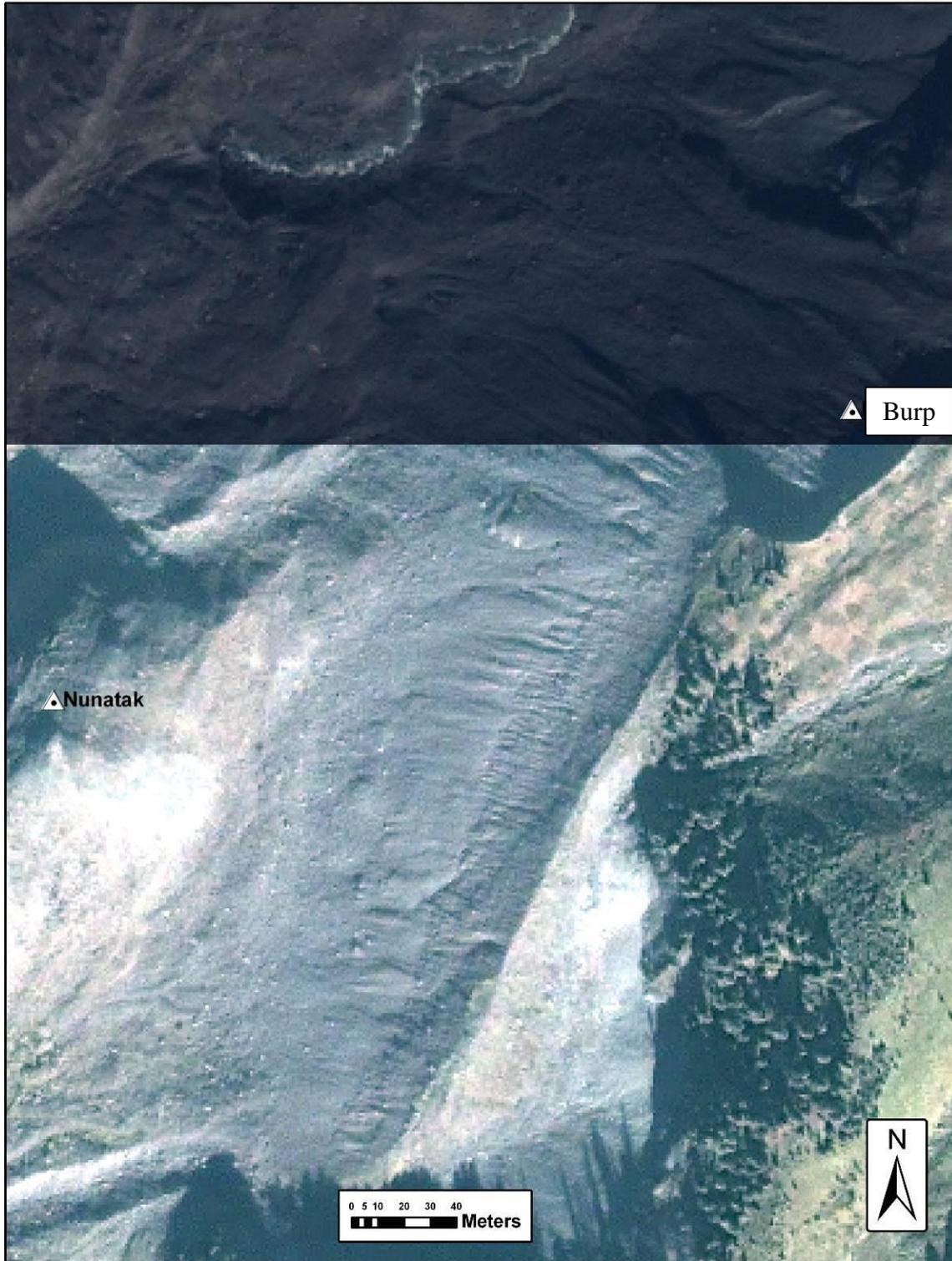
Figure SOP 11.11. Photo identifiable ground control points “Burp” and “Nunatak” surrounding Nisqually Glacier.
