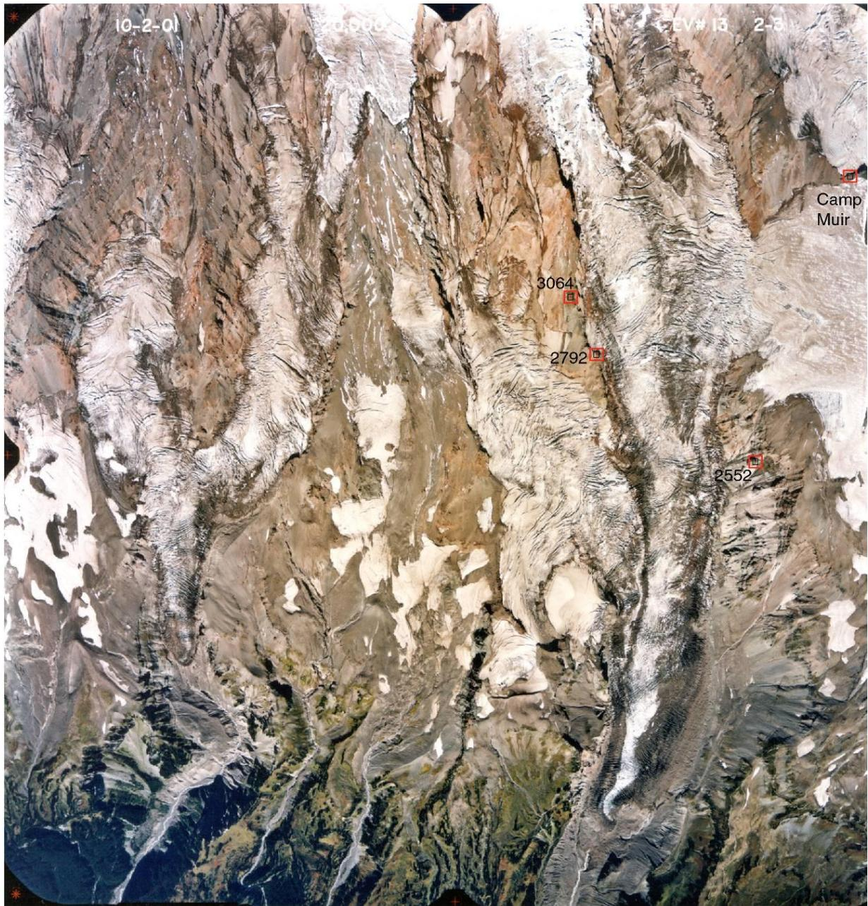
Figure SOP 11.3. Photo identifiable ground control points surrounding Nisqually Glacier.
