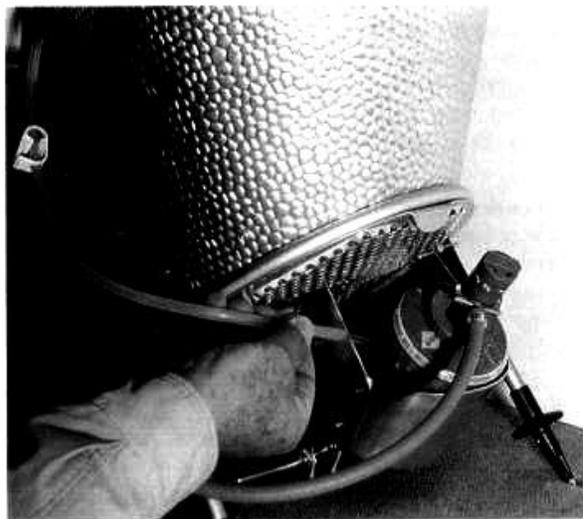
In order to avoid this effect, cartridges are brought to temperature by filling warm water (20 to 40°C, 70 to 100°F) into the cartridge container (15). You can draw warm water, e.g., from the circular bowl via the small drainage hose (illustration at right) or it can come from a thermos flask you have taken with you.
