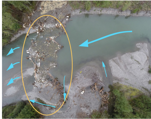
Fig. 7 Channel-spanning ELJs in Upper South Fork Nooksack river, Skagit County, WA.
