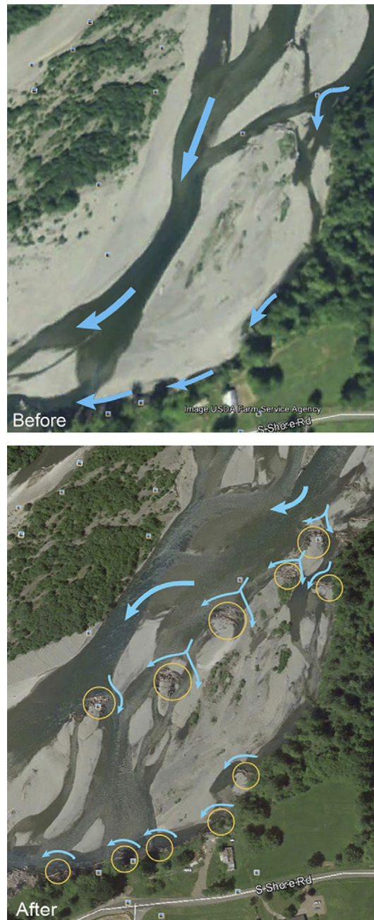
Fig. 5 Preproject (before) and postproject (after) conditions at south shore road Upper Quinault River, Grays Harbor County, WA (this site is downstream of site in Figure 4 and in different county).
