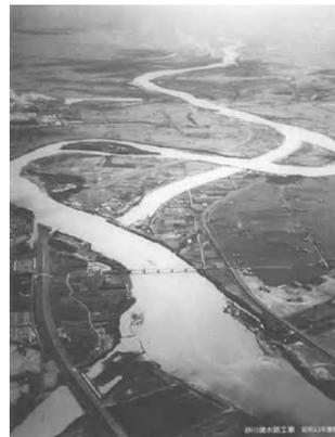
**Figure 13.5** Geomorphic effects of channelisation. (a) Flow and sediment conveyance are greatly enhanced in more uniform, straighter channels. (b) The Ishikari River, near Sapporo, Japan, was channelised to drain a swamp and provide flood protection for development of agricultural land through construction of a hydraulically efficient, low-sinuosity, enlarged channel. (a) Modified from Corning (1975). (b) Photographs provided by Tomomi Marutani.
